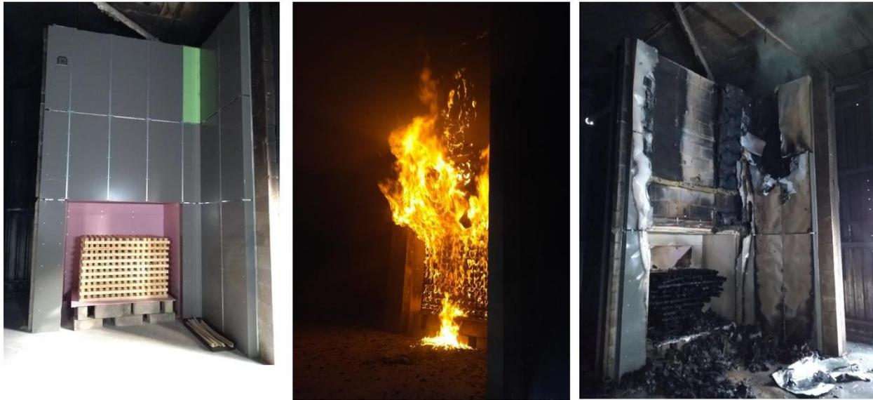
Figure 4 - PIR insulated system with A2 ACM panels
