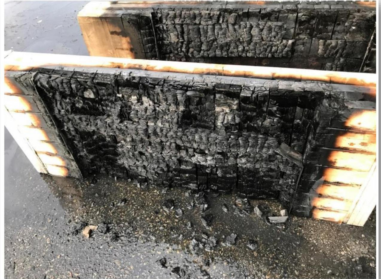
*Delamination of Cross-laminated timber and its impact on fire development Focusing on different types of adhesives, Eric Johansson, Anton Svenningsson - 2018*
