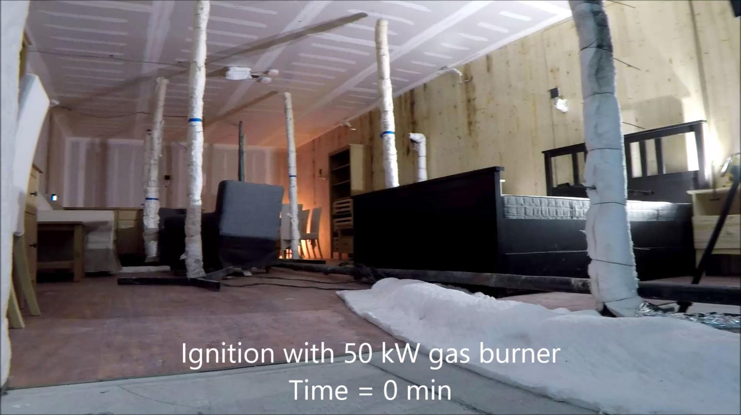
Ignition with 50 kW gas burner
