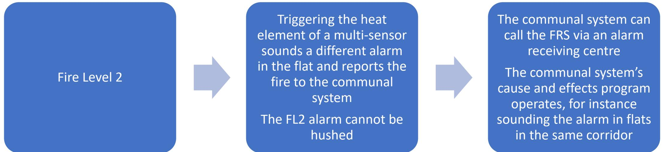
Installing a heat detector in the kitchen and multi-sensors in every other room will give the highest degree of false alarm resistance with the greatest certainty of fast operation in a real fire
