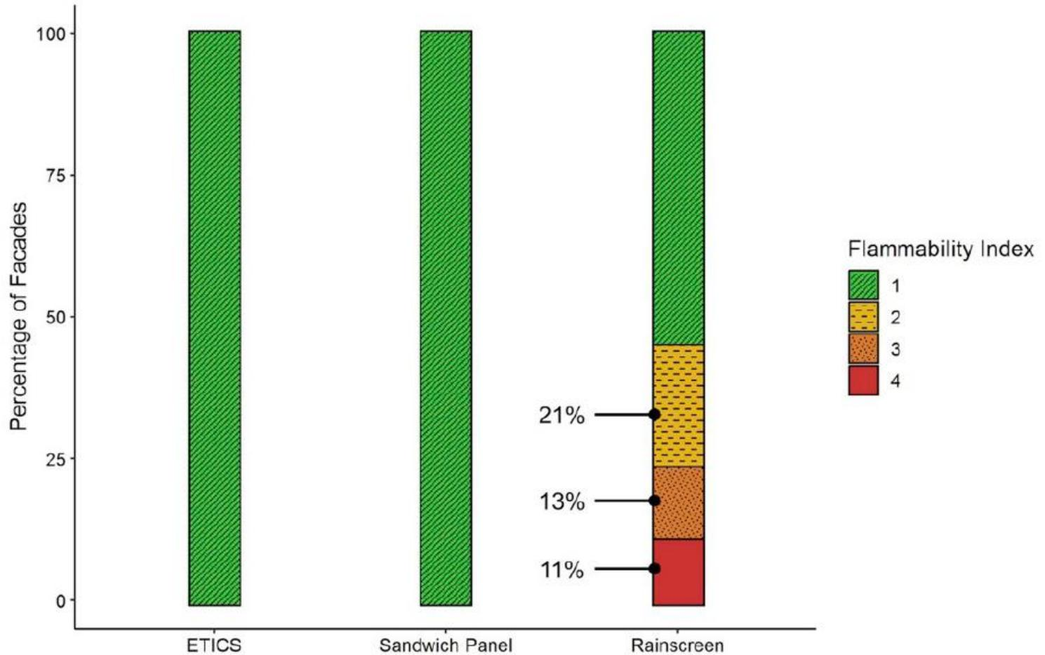
**Fig. 7.** Bar plot of the percentage of facades that fail for different facade types. There were a total of 24 ETICS, 21 Sandwich Panels, and 38 Rainscreen facades
