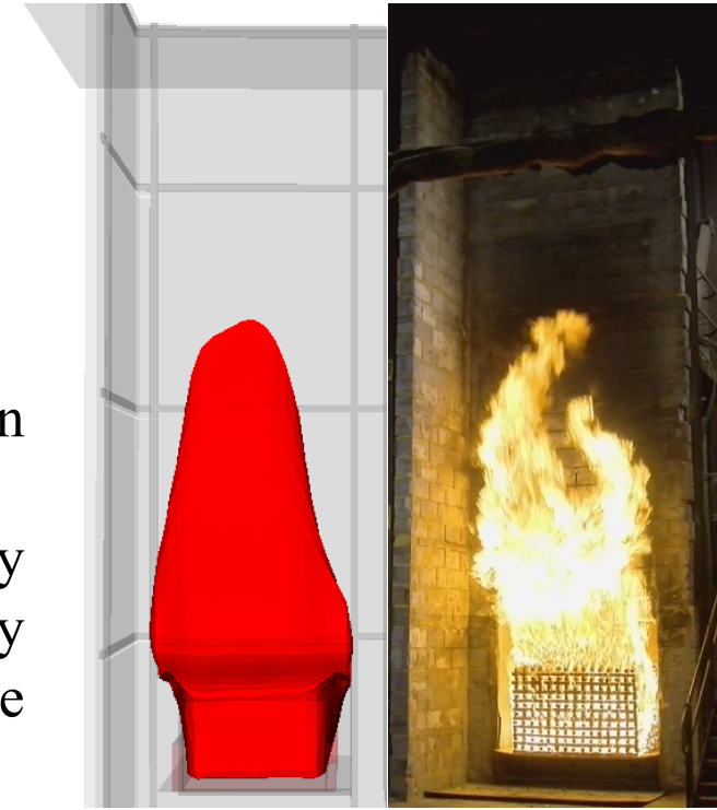
Simulated crib fire plume (525 °C) with a HRR of 2.5 MW and a test without a cladding system
