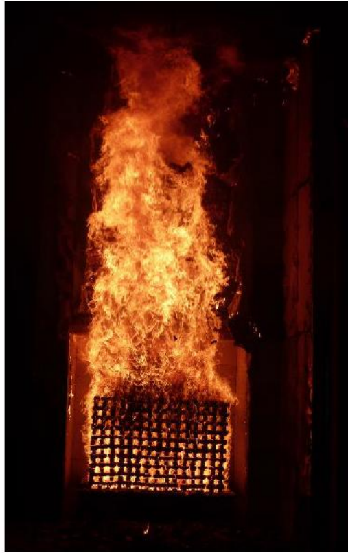
Figure 5 - Phenolic insulated system with A2 ACM panels
