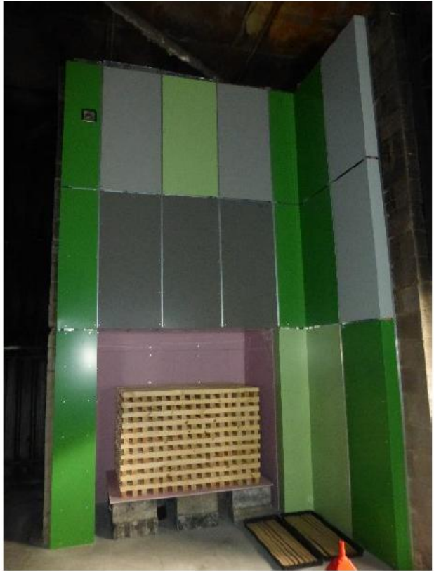
Figure 5 - Phenolic insulated system with A2 ACM panels
