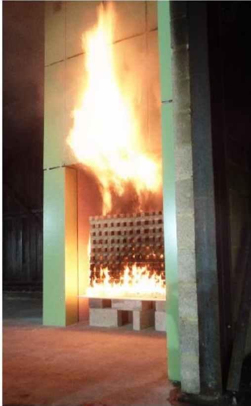
Figure 3 - Stone wool insulated system with A2 ACM panels
