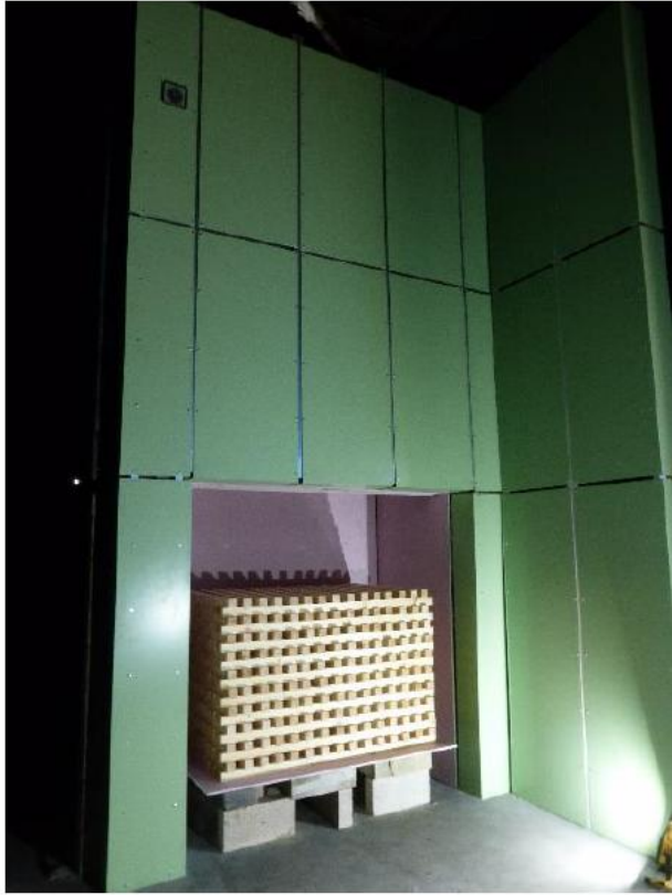
Figure 3 - Stone wool insulated system with A2 ACM panels
