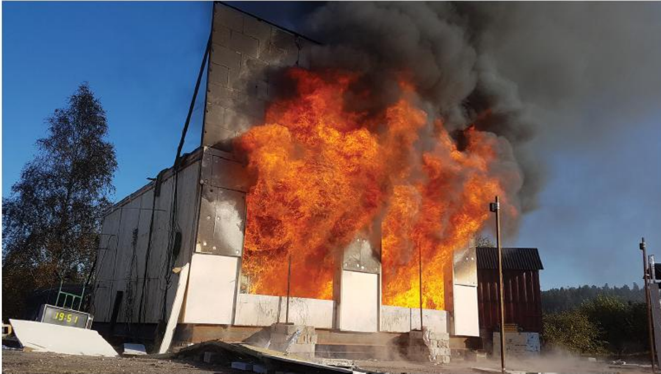
Figure 1 The two-story testing wall exposed to flaming at temperatures over 1600 °F.
