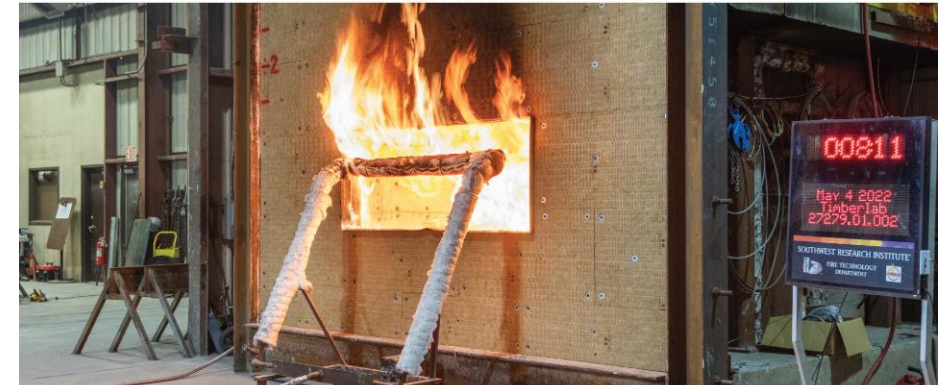
The two-story testing wall exposed to flaming at temperatures over 1600 °F. Courtesy photo by Erika Edwards.
