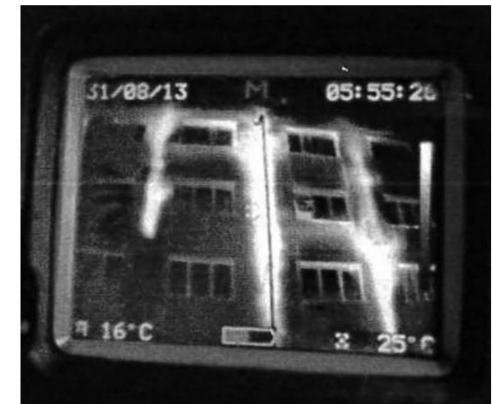
Figure 14.12 Thermal imaging used to identify the extent of fire travel within voids in a burning building (Björkman, 2013; Östman and Stehn, 2014).
