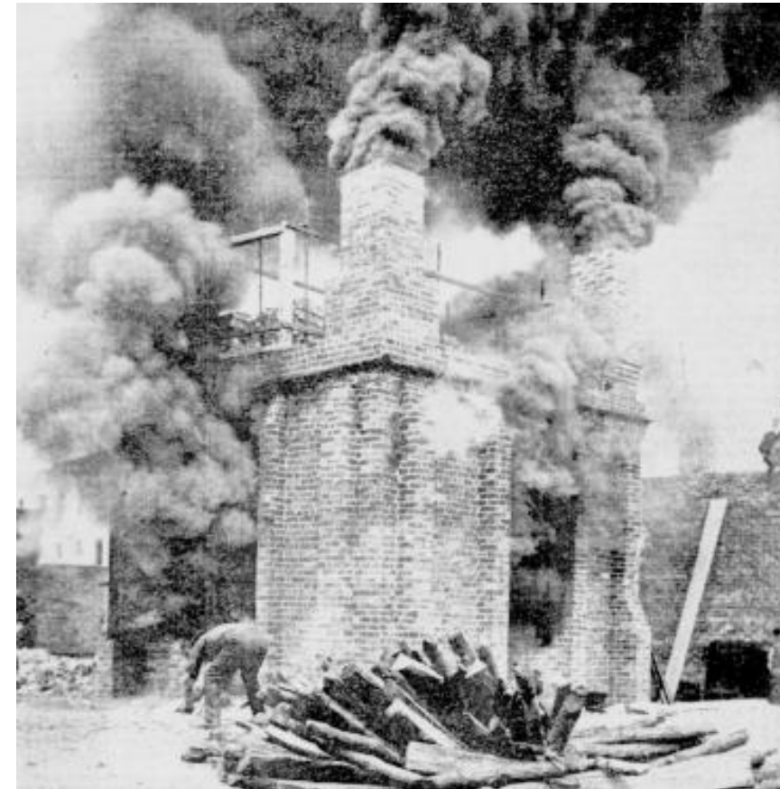
Building department experts applying the fire test to alleged fireproof building materials
